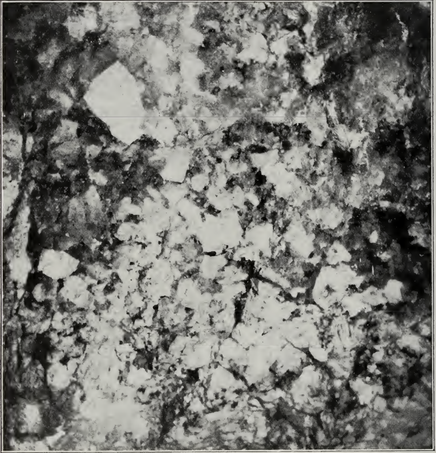
FIG. 23. Mixture of calcite and fluorite 650 feet north of the shaft cross-cut, 350-foot level of the Hillside mine. Note the sharp, straight crystal faces of calcite (light) against fluorite (dark). The largest calcite crystal is three inches in diameter. The calcite of such crystals obviously has not been attacked by fluorite-bearing solutions or the crystal faces would have been impaired.
